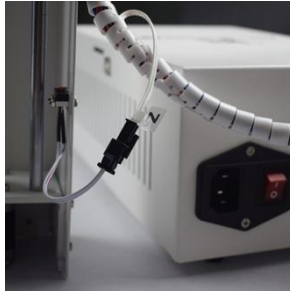
Z axis limit switch with cable (at the lower left of x axis mount )
