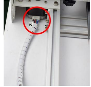
Z axis motor cable (on the left side)
