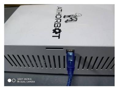
Connect your computer and the 3D printer control box with the USB cable.
