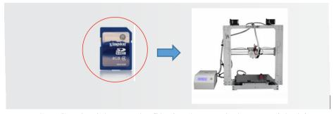
Insert SD Card with .gcode file in the card slot provided in Athorbot control box.
